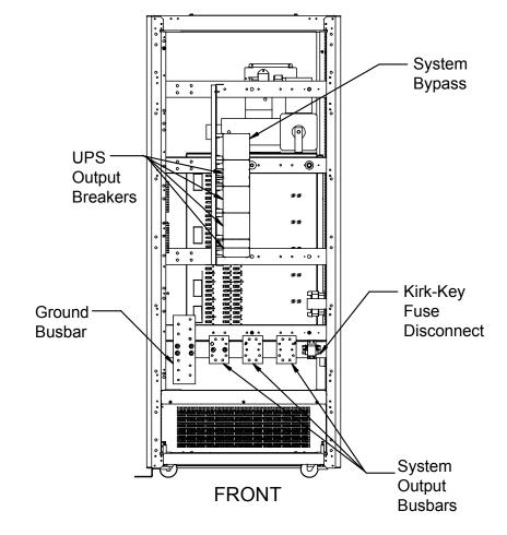
Figure 46 Main component location drawing Liebert<sup>®</sup> NX<sup>™</sup> 480V, CB2, CB3, CB4 configurations
